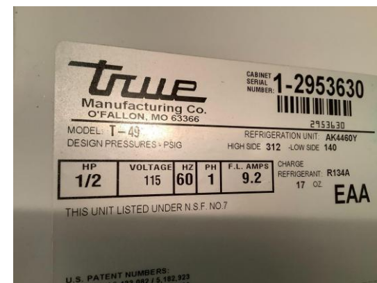
E5 — The label for the kitchen True refrigerator. The serial number suggests it was manufactured in 2000 or 2001, though the database we use stated it couldn't be certain.
